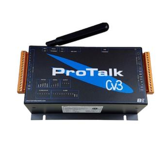
The ProTalk Cv3 provides advanced notification of potentially problematic situations with your site and/or equipment. Capable of monitoring both digital and analog inputs, the ProTalk Cv3 provides versatility and flexibility. The unit is integrated with an LTE cellular module allowing for installation in remote sites. Alarm notifications can be sent via phone, text, email, radio or PA System. Remote alarm acknowledgment, system interrogation and relay control is possible via phone and text.
