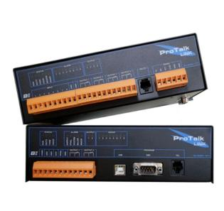
The ProTalk Link provides a flexible, effective solution to a wide variety of alarm monitoring situations. Each system consists of one main module and at least one communication module. The systems can be further expanded using any combination of the available digital, analog or PLC expansion modules. Alarm notifications can be sent via phone, text, email, radio or PA system. Remote alarm acknowledgement, system interrogation and relay control is possible via phone and text.
